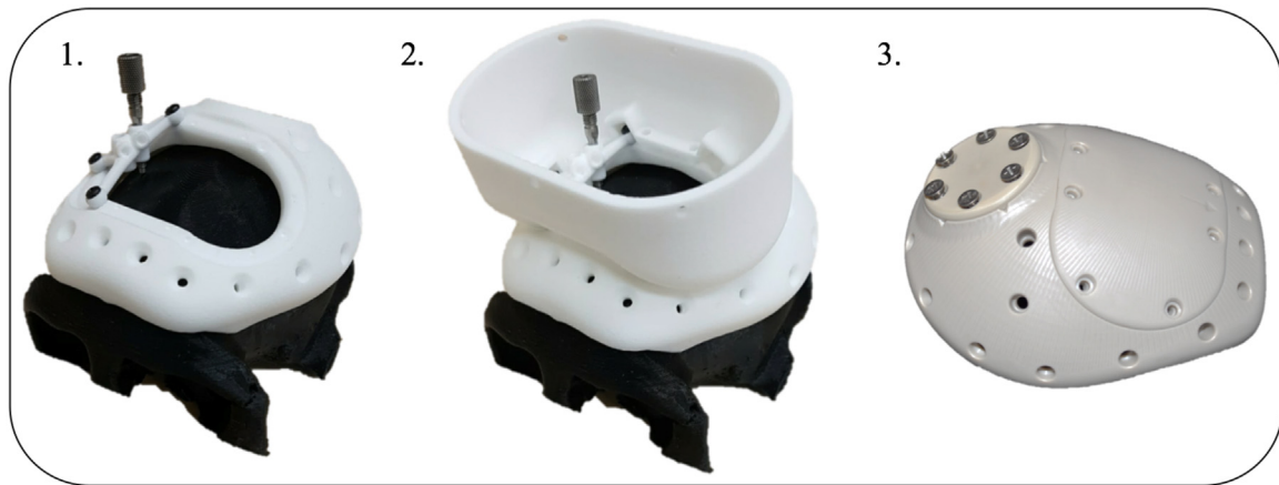
Fig. 9. NHP M cap implant design. (1, 2) 3D-printed prototype and model skull to verify the fit and functionality of the implant. (3) Final PEEK implant with front panel in place.
